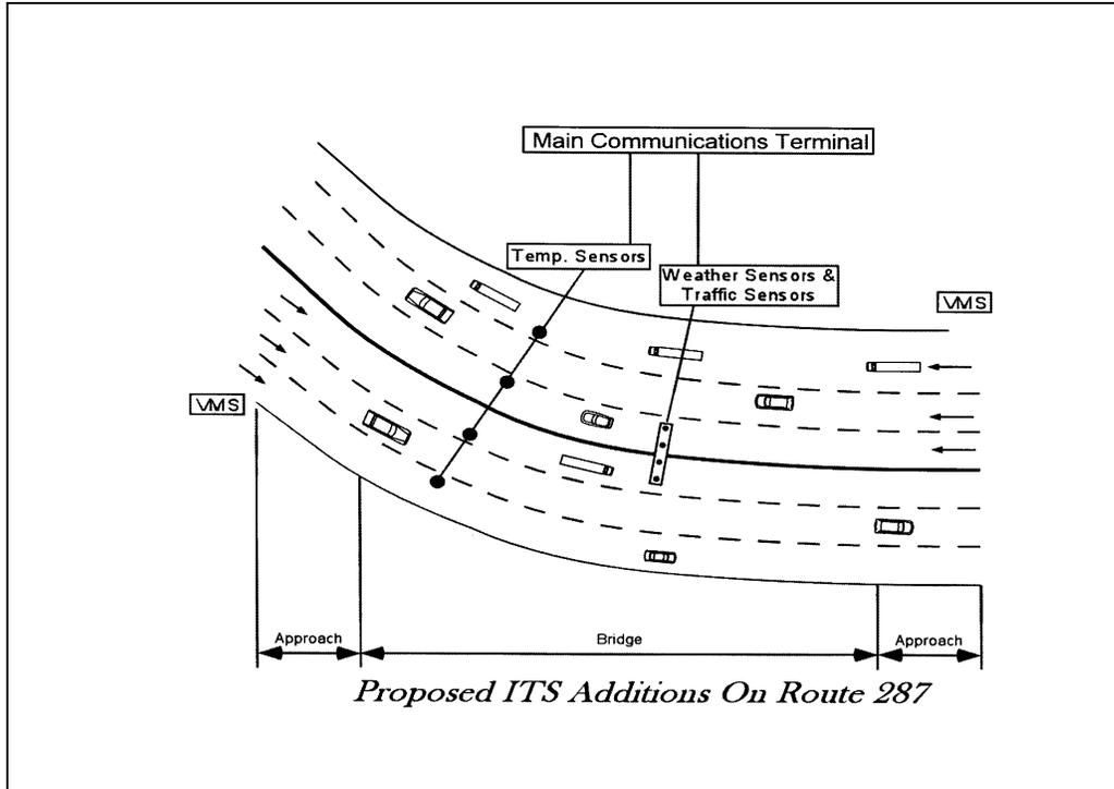
Figure 2. Schematic of the Proposed Weather System for Wanaque Bridge
